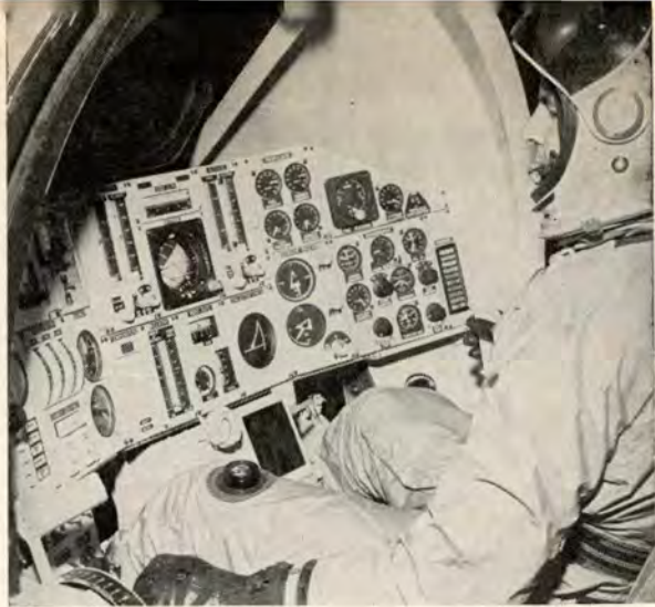
Major John Prodan operates the complex controls of the T-27 Space Flight Simulator at the Aerospace Research Pilot School.
