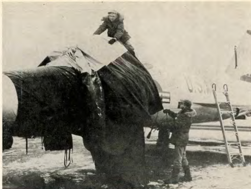
Some aircraft have overcoats which protect surfaces from ice and snow.
